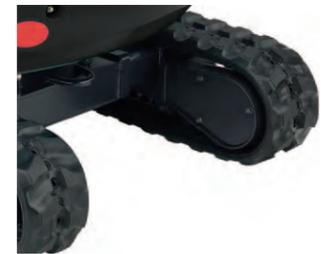
Travel motor hoses are enclosed within the track frame for additional protection. As a result, it reduces repair cost and increases durability.
